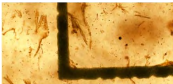
Step 11. Bringing the grid lines on the McMaster slide into focus.
